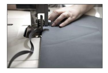
**Ultrasonic sewing**: advanced manufacturing technique to join synthetic materials by using ultrasonic waves to create heat and weld together the fabric's fibers for a sew less connection.
