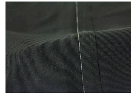
Protected and hidden seam. / LD100 cover tape
